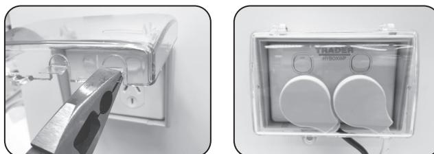
If using the assembly with plugs that are required to be inserted for permanent applications it is best to break out the lower tabs to allow cable clearance and utilise side entry plugs so that the flap can remain closed for maximum protection.
