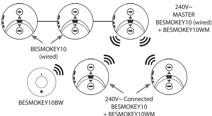
BESMOKEYREM can be installed on wireless network for convenient control.
