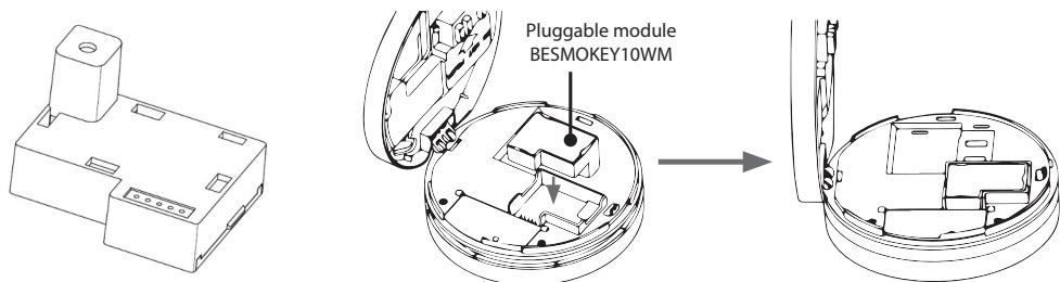
To make wireless, before removing battery tag add BESMOKEY10MW, then connect battery and power. Follow instruction to pair the wireless alarms in the network.
